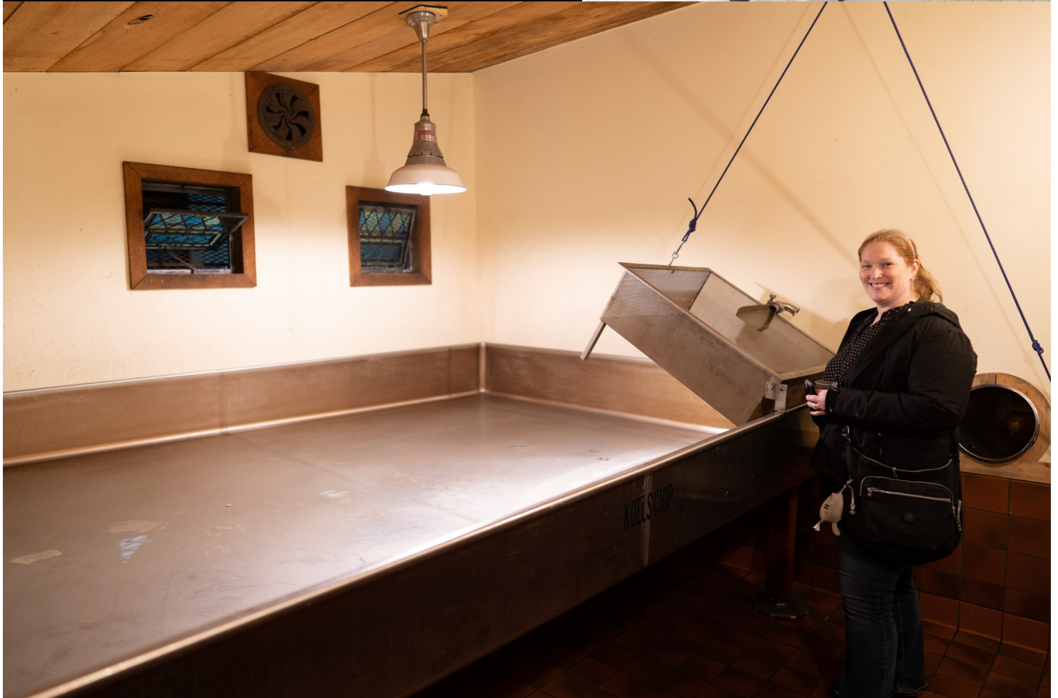
Allagash Brewing Company's Coolship, an open-air fermenter used to make spontaneously fermented beer, was the first in the US
